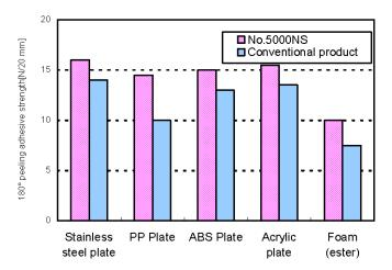
(Unit: N/20mm) Sample width: 20 mm Backing material: PET#25 Application condition:
