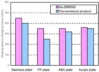
(Unit: N/20mmx20mm) Sample: 20mm x 20mm Pressure condition: 49N load x 10 sec Bonding temperature: 23degreeC/50%RH Curing condition: 23degreeC/50%RH x 30 min No.5000NS Measurement condition: 23degreeC/50% RH Tensile direction
