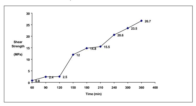
After 24 hrs : 33.3 MPa After 48 hrs : 36.6 MPa After 96 hrs : 37.9 MPa After 7 days : 36.5 MPa After 15 days : 39.3 MPa After 30 days : 36.2 MPa After 60 days : 35.8 MPa
